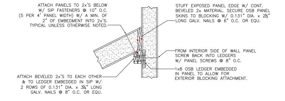
NOTE: ALL RED DOTS — APPLY CONTINUOUS 3/8" DIA. BEAD OF MASTIC SEALANT BETWEEN 2x MEMBER & PANEL FOAM.
