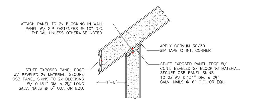
NOTE: ALL RED DOTS — APPLY CONTINUOUS 3/6" DIA. BEAD OF MASTIC SEALANT BETWEEN 2x MEMBER & PANEL FOAM.
