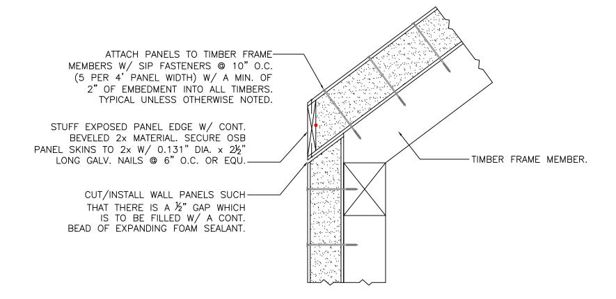
NOTE: ALL RED DOTS — APPLY CONTINUOUS 3/8" DIA. BEAD OF MASTIC SEALANT BETWEEN 2x MEMBER & PANEL FOAM.
