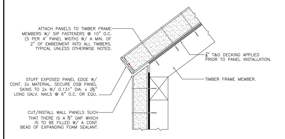
NOTE: ALL RED DOTS — APPLY CONTINUOUS 3/6" DIA. BEAD OF MASTIC SEALANT BETWEEN 2x MEMBER & PANEL FOAM.
