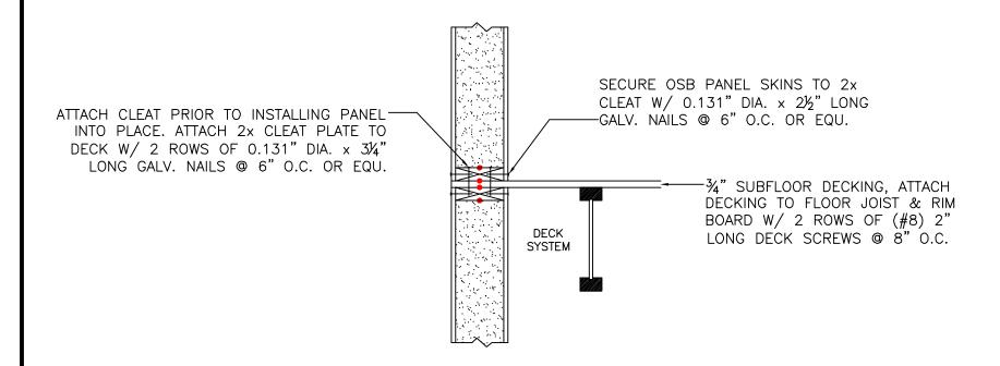
NOTE: ALL RED DOTS — APPLY CONTINUOUS 3/8" DIA. BEAD OF MASTIC SEALANT BETWEEN 2x MEMBER & PANEL FOAM.
