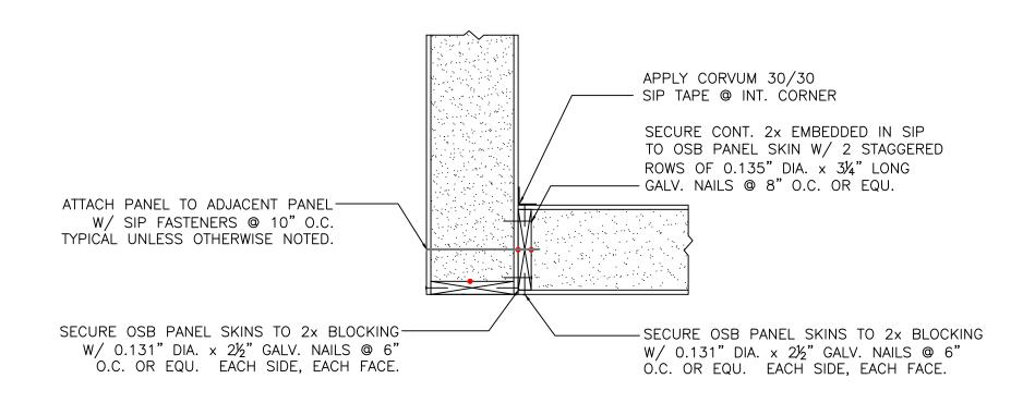
NOTE: ALL RED DOTS — APPLY CONTINUOUS 3/8" DIA. BEAD OF MASTIC SEALANT BETWEEN 2× MEMBER & PANEL FOAM.
